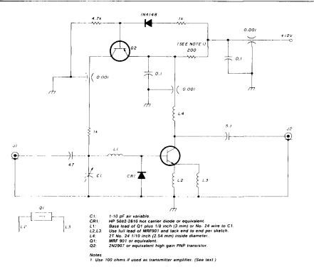
fig. 6. A simple low noise preamplifier for a 33 cm receive type converter. Gain is approximately 12 dB and noise figure is 2.5-3 dB typical. If the 200 ohm resistor in the constant current source is changed to 100 ohms, it will function well as a low-level linear transmitter amplifier stage as discussed in text.
